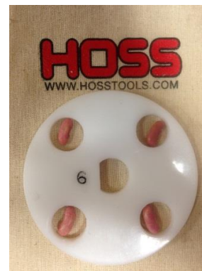
Seed Plate #6 with Contender Green Beans. Holes have been drilled large enough so that bean seeds lay flat in the holes and can easily fall through the plate.
