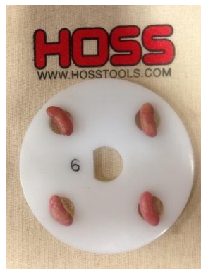
Seed Plate #6 with Contender Green Beans. Notice the holes in the plate are too small and will need to be drilled larger.
